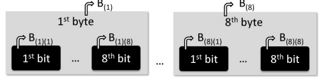
Figure 1 Representation of a cryptographic key where B_{(j)(i)} represents the i -th bit of the j -th byte of the (sub)key.
